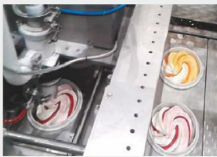
3-axial servo-driven dosing unit
