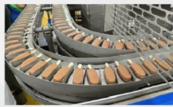
Two pocketed conveyors, special version angular (90 degree)
