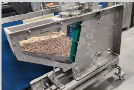
Automatic stick inserter - unit allowing work with loose sticks, not arranged in stacks with banderole
