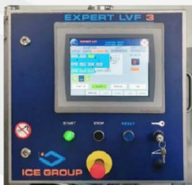
Operator friendly, full-colour touch-screen panel for control and synchronization of particular elements of the line
