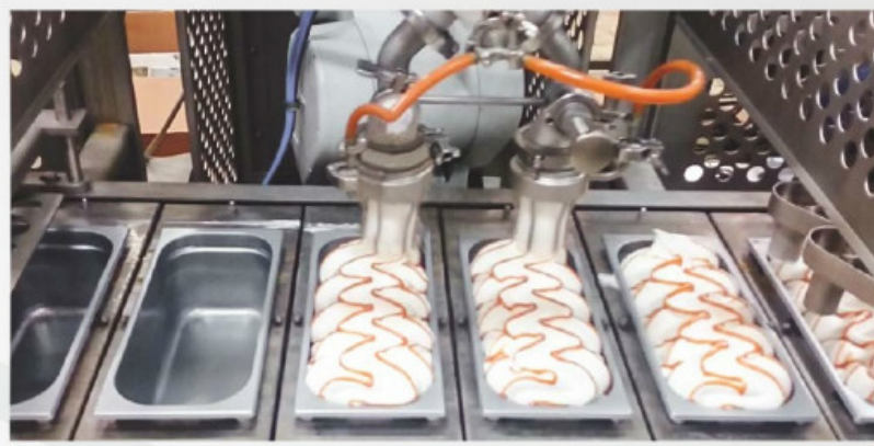
Two tubs simultaneous dosing to maximize capacity
