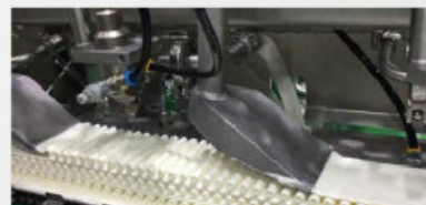
Version with reel paper dispenser, from which the tray is formed - the product is automatically cut together with the tray by means of a mechanically actuated knife
