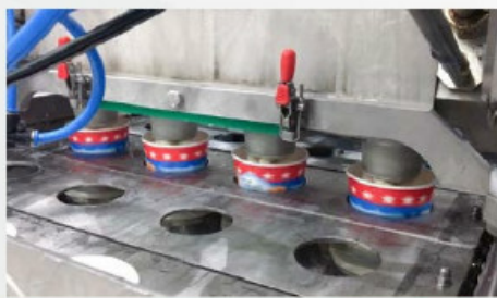
Volumetric dosing unit enables dosing low overrun, high viscose ice cream with extra large inclusions.
