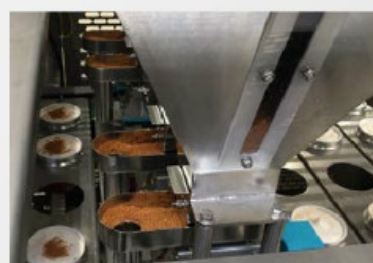
Vibration dry ingredient dosing unit
