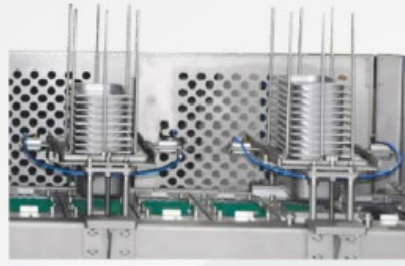
Automatic 5-liter tubs destacking station
