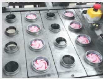
4-wide machine for Ø75mm and Ø95mm cups - Double Pitch version
