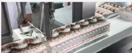
Version with reel paper dispenser, from which the tray is formed - the product is automatically cut together with the tray by means of a mechanically actuated knife
