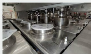
Sealing station for aluminium, paper or plastic lids
