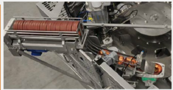
Special dispensing station for unstackable paper or plastic lids.
