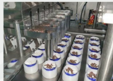
Vibration dry ingredient dosing unit
