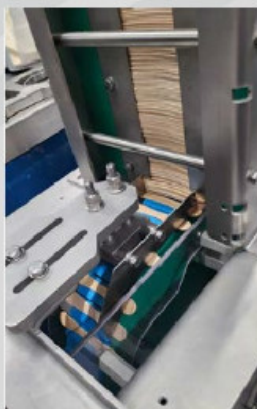
Automatic stick inserter - unit allowing work with loose sticks, not arranged in stacks with banderole
