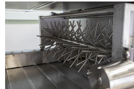
Adjustable spike roller gently separates coated products
