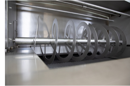
Helical spreader ensures level product bed
